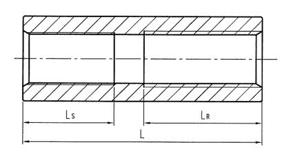
Ls: length of thread for threadbar Ls: length of thread for plain bar
