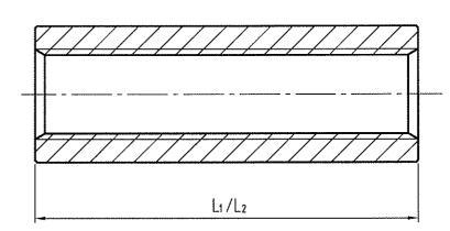
$L_1$ : length of coupler 3003  $L_2$ : length of coupler L 3303 (coupler L for unbonded tendon with angular cut threadbars)
